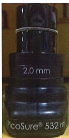
2.0mm Spacer for 532nm LDS
